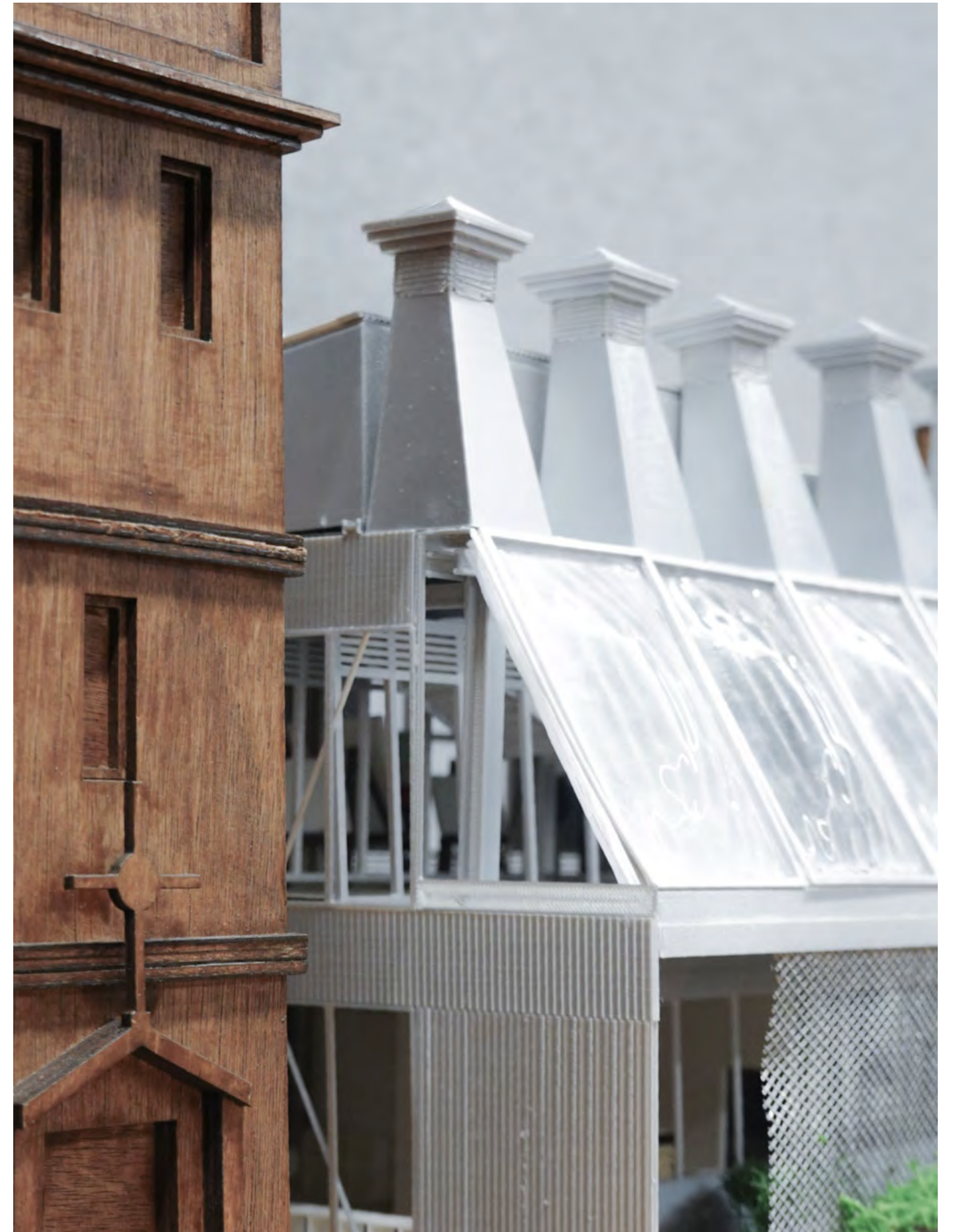
Fig.20. solar chimney and buffer zone
